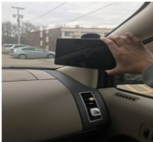
Step 3: Tablet is attached onto The A-pillar.
