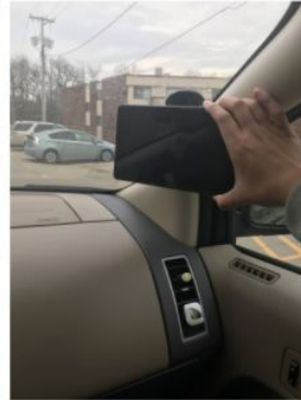
Step 3: Tablet is attached onto The A-pillar.
